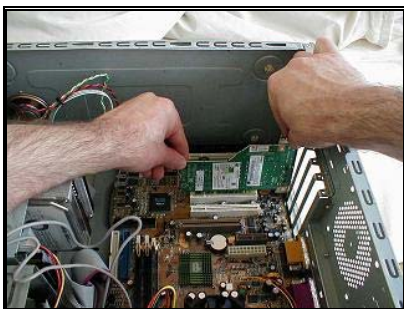
Figure 4: Mounting the video card into the slot
